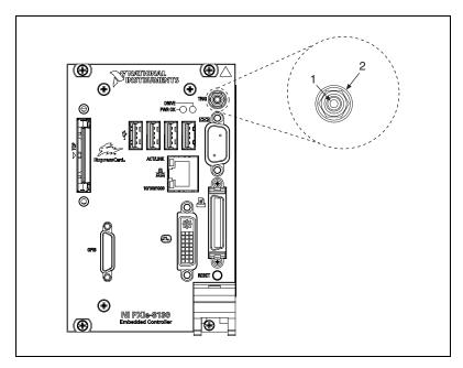
Figure 3-7. TRIG Connector Location and Pinout
